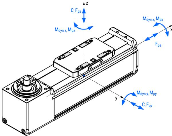
The moved mass is already considered in the equation for calculating the mass of the linear unit  $m_{MGTB}$  and the mass moment of inertia  $J_{MGTB}$ . The moved mass includes the mass of the carriage.
